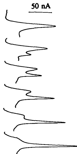
Fig 1 Voltammograms of 0.2 \mu\text{M} PCV containing 0, 20, 40, 60, 80, and 100nM V, 20mM acetate buffer, preconcentration for 60 sec, scan rate of 0.05 V/sec
